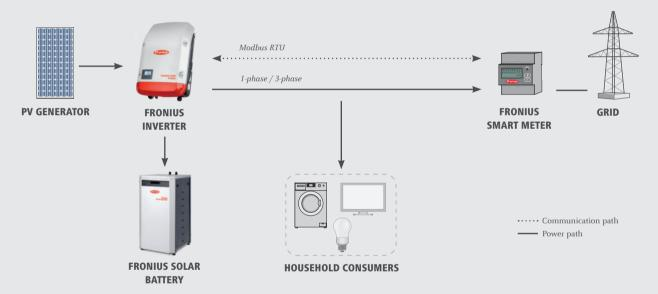
/ The Fronius Smart Meter is compatible with all inverters with an RS485 interface (Modbus RTU). The Fronius Smart Meter works in conjunction with the Fronius Datamanager 2.0 for the Fronius IG Plus and Fronius CL inverters, whereas the Fronius Datamanager Box 2.0 is used with the Fronius IG TL, Fronius Agilo and Fronius Agilo TL inverters. The Fronius Smart Meter can be retrofitted at any time together with the Fronius Datamanager 2.0 in inverters that have already been installed.
